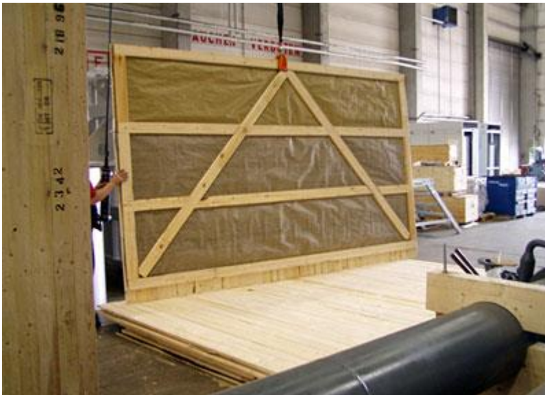
Figure 7: Side wall lined with a barrier layer
