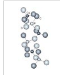
Crystal structure of Gallium Orthophosphate.
