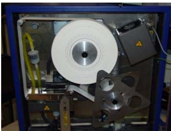
Fig. 24 Inside the device, the paper transport mechanism
