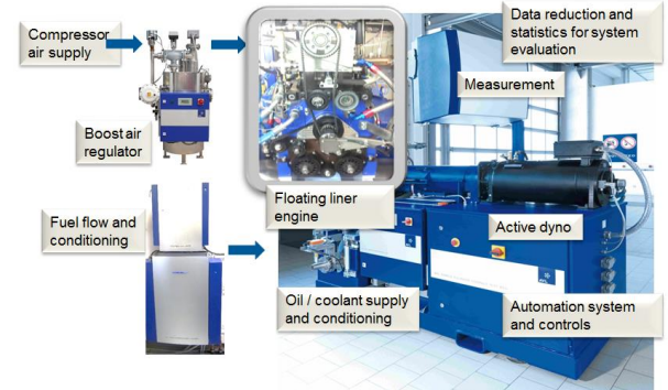
Figure 12: The floating liner engine is part of a test bed system comprising modules to enable precisely defined engine operation and measurement.
